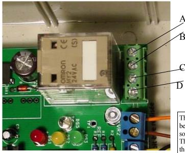
Open dry contacts that close on power for connection to Boiler TT
